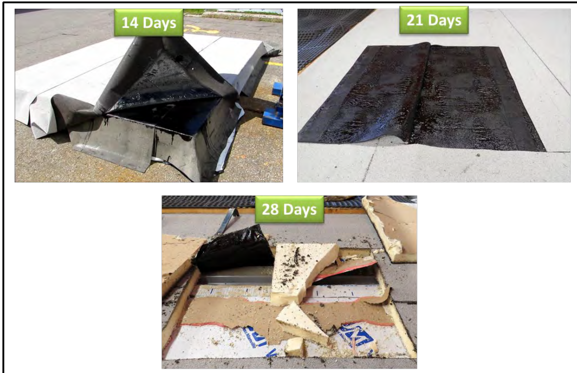
Figure 16: Failure modes varied with curing time for AARS
