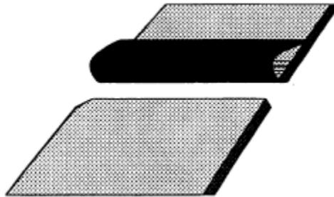
Granule end laps should be prepared well before the following roll approaches for bonding to the end lap. If granule embedment is delayed until the next roll is within 600 mm (24") of the end lap, the rolled material will overheat from residual heat generated from the embedding process.
